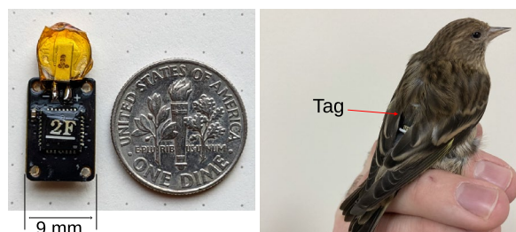
Fig. 1 BitTag. Left image shows the top side of a BitTag with a 0.23 g, 5.5 mA h battery. Right image shows a Pine Siskin (12–18 g) with tag. Tags are attached with a loop harness [39] constructed from elastic thread. Pine Siskin photo courtesy of Ben Vernasco
