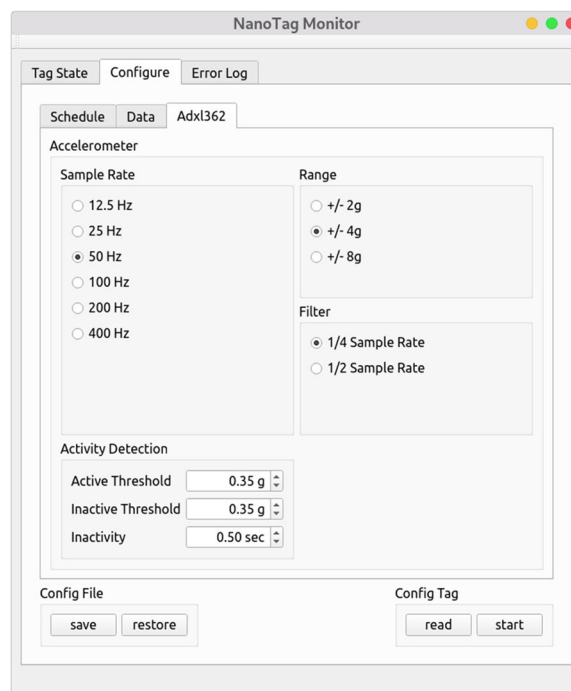
Fig. 13 qtmonitor adxl362 configuration tab. The BitTag configuration provides a number of options for the ADXL362 accelerometer. The most important configurations are the activity detector thresholds and inactivity delay. In addition, the accelerometer sample rate (when active) can be configured along with the range. These configurations are provided to enable support for custom firmware—in the case of BitTag the defaults are generally accepted
