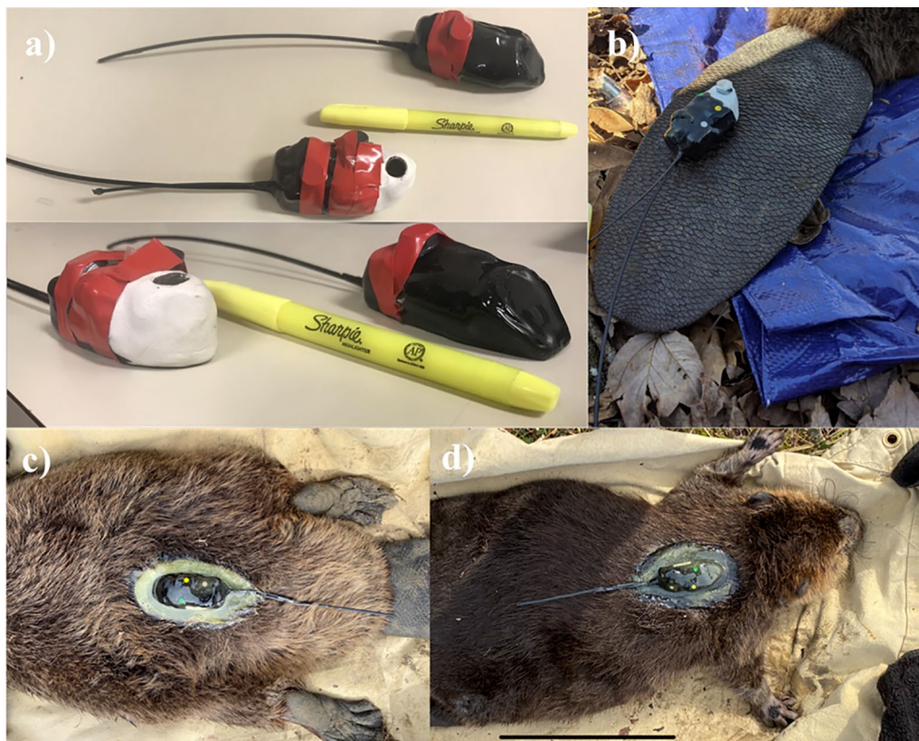
Fig. 1 Picture including custom-designed transmitters and various attachment methods. Pictures displaying a the customized tail-mount (transmitter with white colored end and hole to facilitate bolting the transmitter to the tail) and back-mount transmitters (the red tape was used to fasten magnets to the transmitters, temporarily disabling the GPS and VHF until deployment), b a tail-mounted transmitter successfully secured to the tail of a captured beaver, c transmitter adhered to the lower back using mid-cure epoxy, and d transmitter adhered to the upper back using mid-cure epoxy
