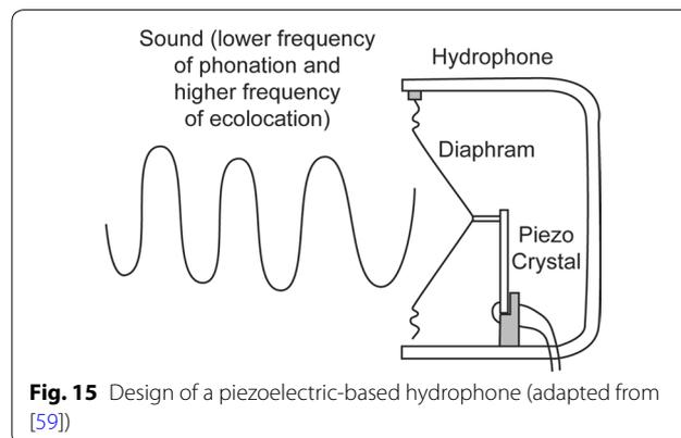
**Fig. 15** Design of a piezoelectric-based hydrophone (adapted from [59])
