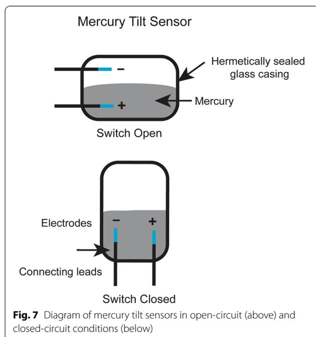
**Fig. 7** Diagram of mercury tilt sensors in open-circuit (above) and closed-circuit conditions (below)
