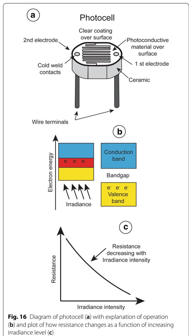
**Fig. 16** Diagram of photocell (a) with explanation of operation (b) and plot of how resistance changes as a function of increasing irradiance level (c)
