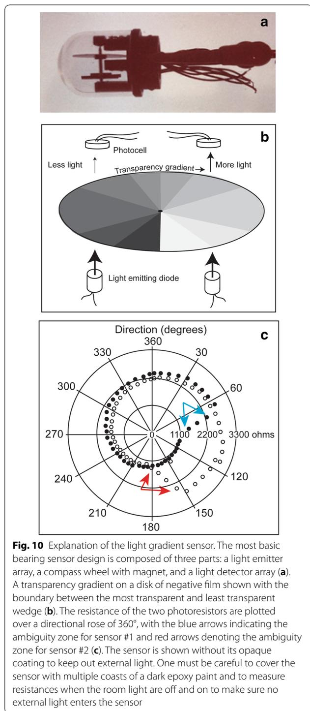
the compass wheel carrying a disk with a transmission gradient (Fig. 10a). This is usually created from a film negative exposed for increasing times to produce a radial transmission gradient (Fig. 10b). The sensor operates by detecting differences in light that correspond to
