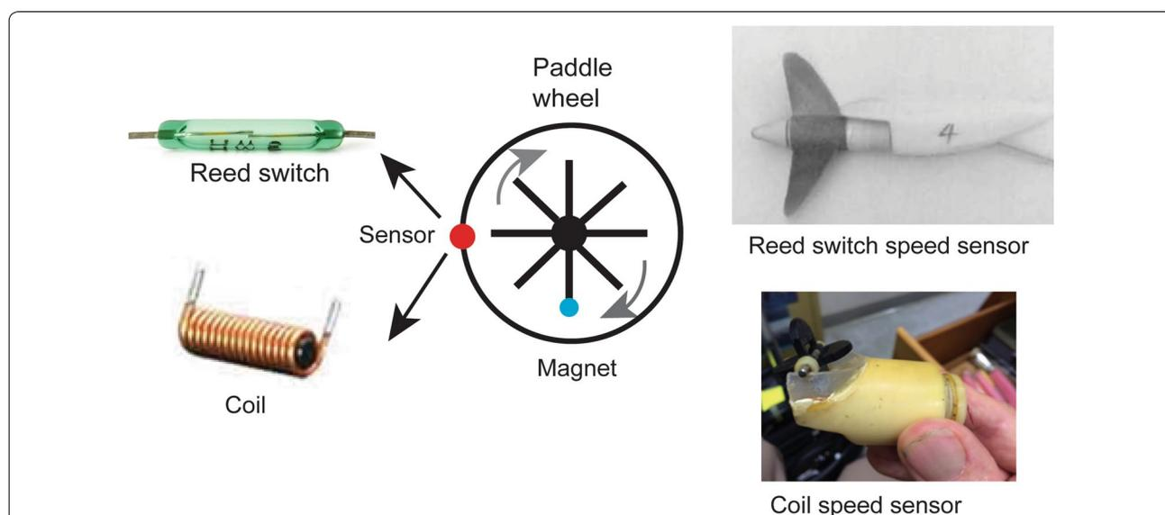
**Fig. 1** Two paddle wheel sensors used to record swimming speed. Pictures of a reed switch and coil (left) and a propellor and paddle wheel sensor with these two components (right). Wheel with magnet in one paddle shown rotating toward the two sensors (center)
