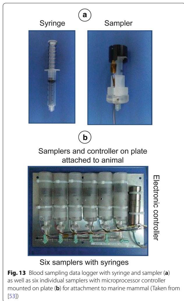
**Fig. 13** Blood sampling data logger with syringe and sampler (a) as well as six individual samplers with microprocessor controller mounted on plate (b) for attachment to marine mammal (Taken from [53])
