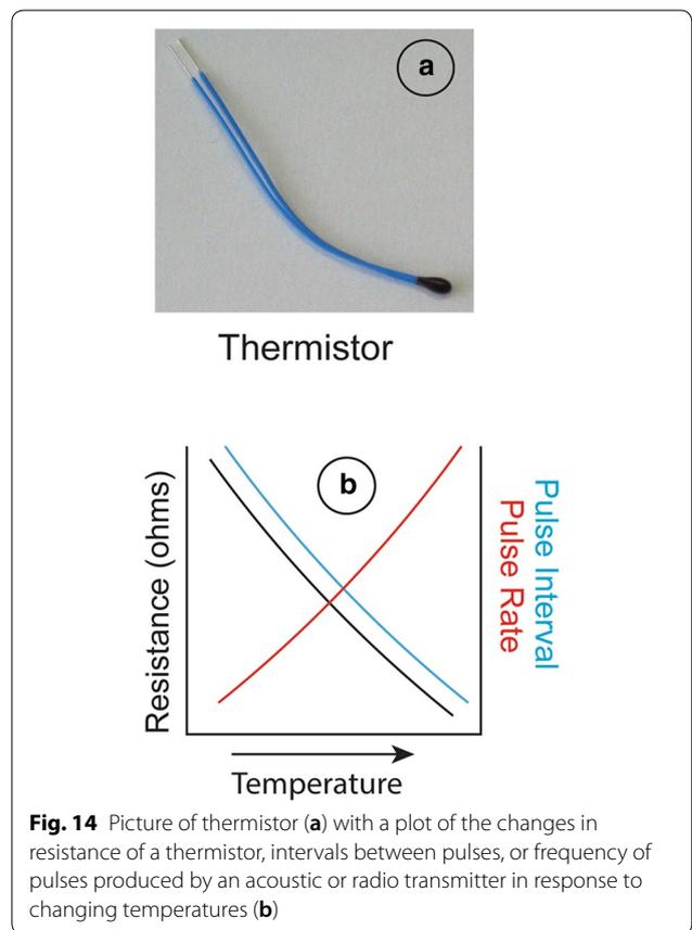
**Fig. 14** Picture of thermistor (a) with a plot of the changes in resistance of a thermistor, intervals between pulses, or frequency of pulses produced by an acoustic or radio transmitter in response to changing temperatures (b)
