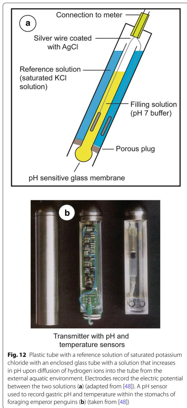
environment diffuse into the glass tube through the permeable distal end and increase the electric potential. The more hydrogen ions that diffuse into the glass tube, the higher the electric potential and lower the pH. The voltage measured between the two electrodes is processed to produce a pH value of the solution.
