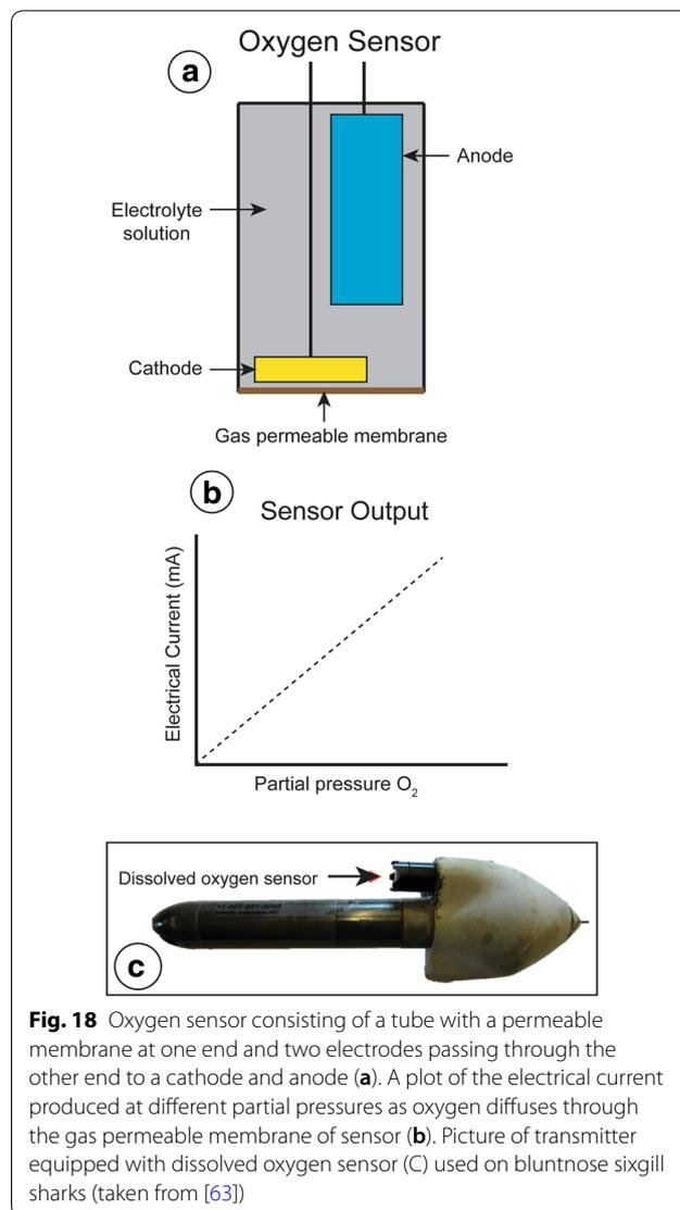
**Fig. 18** Oxygen sensor consisting of a tube with a permeable membrane at one end and two electrodes passing through the other end to a cathode and anode (a). A plot of the electrical current produced at different partial pressures as oxygen diffuses through the gas permeable membrane of sensor (b). Picture of transmitter equipped with dissolved oxygen sensor (c) used on bluntnose sixgill sharks (taken from [63])
