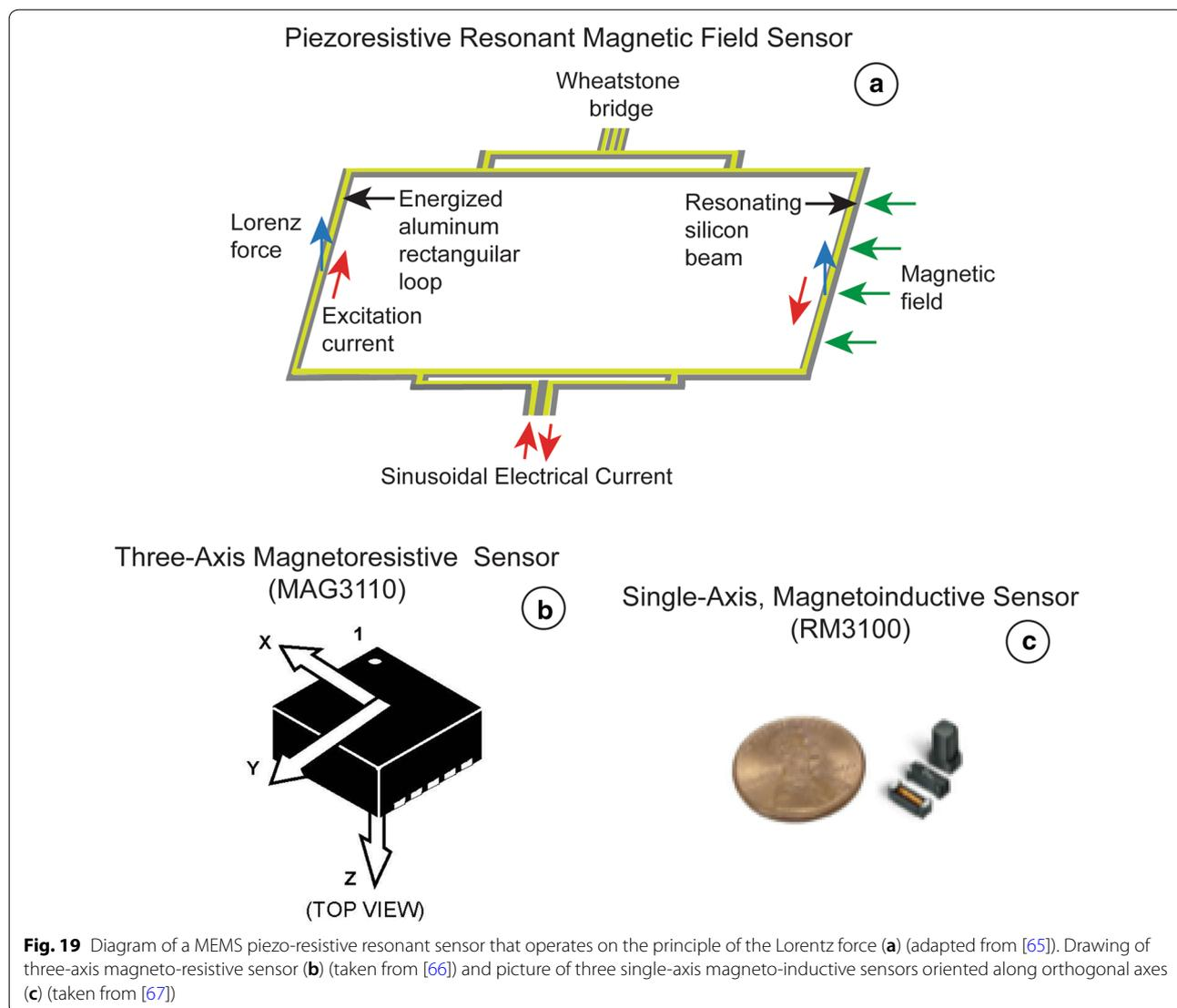
**Fig. 19** Diagram of a MEMS piezo-resistive resonant sensor that operates on the principle of the Lorentz force (a) (adapted from [65]). Drawing of three-axis magneto-resistive sensor (b) (taken from [66]) and picture of three single-axis magneto-inductive sensors oriented along orthogonal axes (c) (taken from [67])
