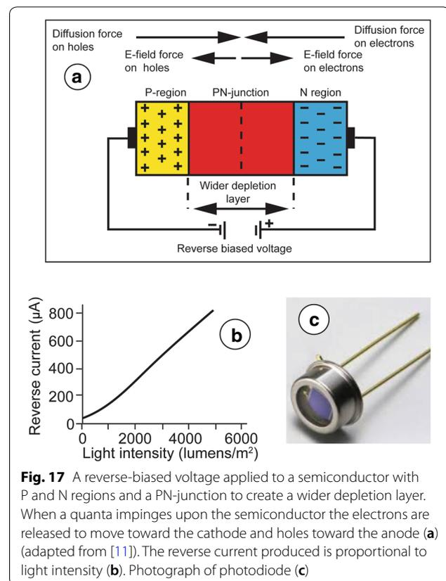
**Fig. 17** A reverse-biased voltage applied to a semiconductor with P and N regions and a PN-junction to create a wider depletion layer. When a quanta impinges upon the semiconductor the electrons are released to move toward the cathode and holes toward the anode (a) (adapted from [11]). The reverse current produced is proportional to light intensity (b). Photograph of photodiode (c)
