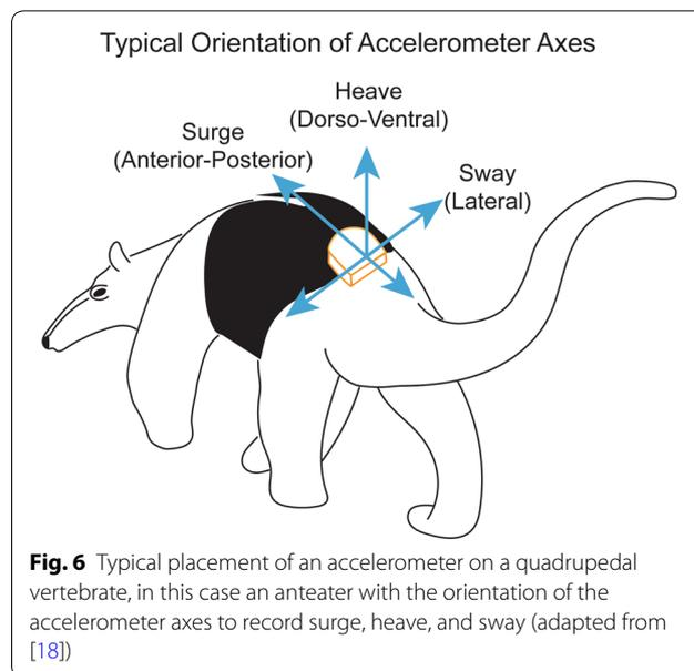
the airplane pilot. The typical orientations of a triaxial accelerometer's axes when deployed on an animal are illustrated on the tamandua, a small anteater (*Tamandua mexicana*) (Fig. 6).
