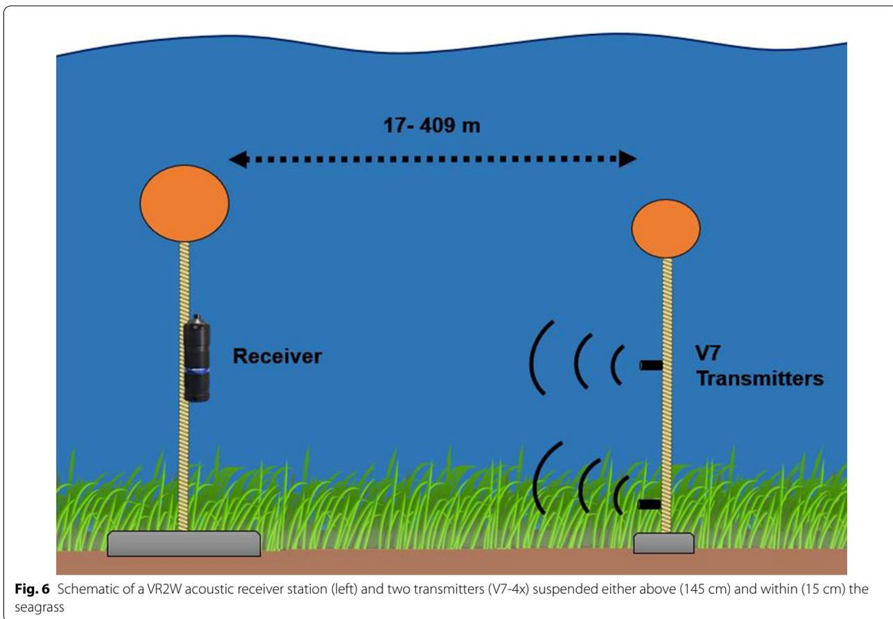
**Fig. 6** Schematic of a VR2W acoustic receiver station (left) and two transmitters (V7-4x) suspended either above (145 cm) and within (15 cm) the seagrass
