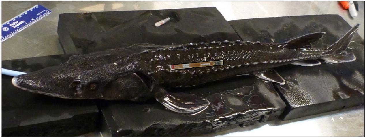
**Fig. 2** Approximate location of the self-powered transmitter (SPT) to maximize energy output from the fish's natural swimming motion. The SPT pictured is overlain the sturgeon in an upright position for visual aid to where the SPT was implanted horizontally between the dermis and hypodermis tissue and is roughly to scale (65 mm in length)
