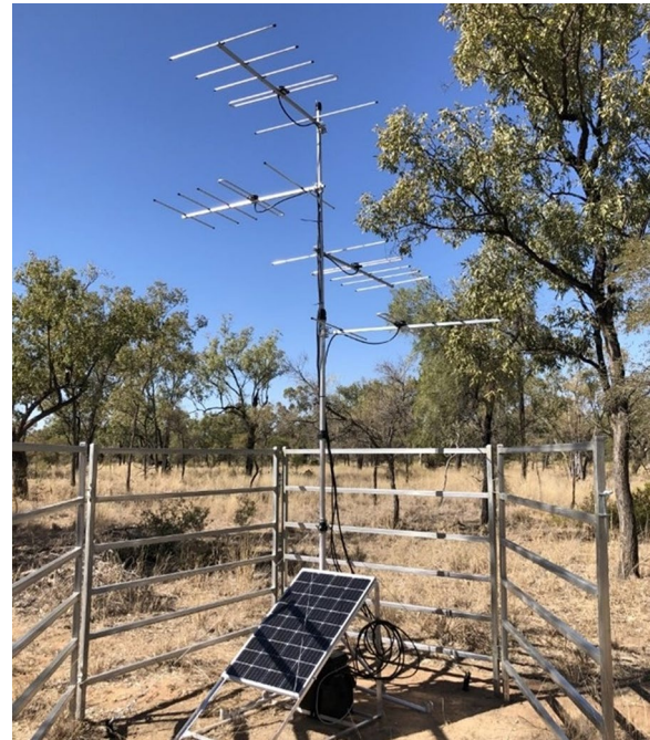
Fig. 3 Automated radio telemetry receiver with four directional antennas installed within the study area
