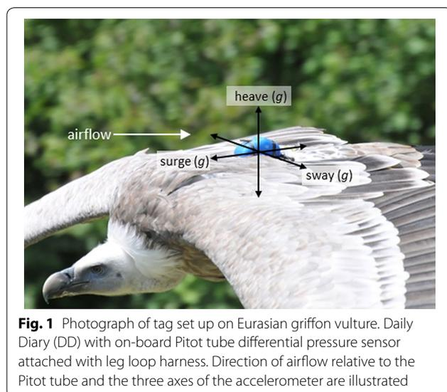
**Fig. 1** Photograph of tag set up on Eurasian griffon vulture. Daily Diary (DD) with on-board Pitot tube differential pressure sensor attached with leg loop harness. Direction of airflow relative to the Pitot tube and the three axes of the accelerometer are illustrated
