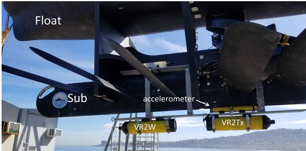
**Fig. 2** Wave Glider SV3 consists of a float and sub connected by a tether. The surface float contains communications, solar panels, batteries and integrated sensors. The sub has wings, a rudder and thruster for propulsion. The photograph shows custom-made steel brackets and plates where the VR2W receiver (forward facing), VR2Tx transceiver (backward facing) and accelerometer were mounted. The front of the vehicle is on the left
